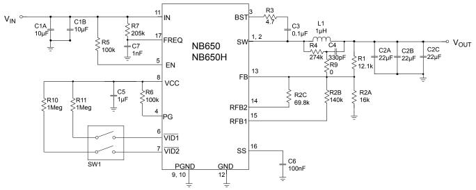
Figure 13: Typical Application with Low-ESR Ceramic Capacitor  $V_{IN} = 12V$ ,  $V_{OUT} = 1.05/1.10/1.15/1.20V$ ,  $I_{OUT} = 6A$ ,  $f_{SW} = 550$ kHz
