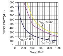
Figure 4: Plot of V<sub>OUT</sub> as a Function of R<sub>FREQ</sub> and the Frequency
