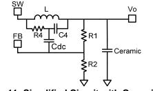
Figure 11: Simplified Circuit with Ceramic DC-Blocking Capacitor
