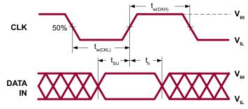
Figure 1: Input Timing Voltage Waveforms
