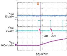
When MP1529 starts up under PWM Dimming mode, the first pulse width of EN1 is required to be more than 8µs to wake up the part. The pulse width can be as low as 2µs after MP1529 is active.
