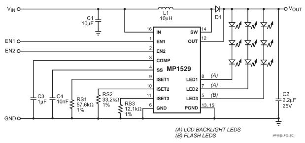
Figure 3—Driving 2 x 3 Backlight Strings (20mA per WLED) and 1 Flash String (40mA Preview, 100mA Flash)
