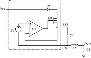
Figure 2—Internal Bootstrap Charging Circuit
