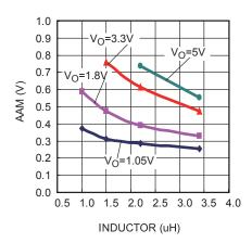
Figure 5— AAM Selection for Common Output Voltages (V<sub>IN</sub>=7V-24V)
