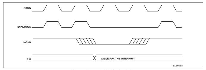
Figure 7. Interrupt Bid Arbitration Timing
