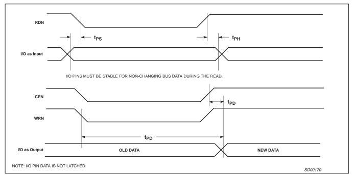
Figure 11. I/O Port Timing
