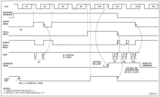
Figure 17. Receiver Data Timing
