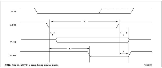
Figure 6. Interrupt Knowledge (IACKN) Timing
