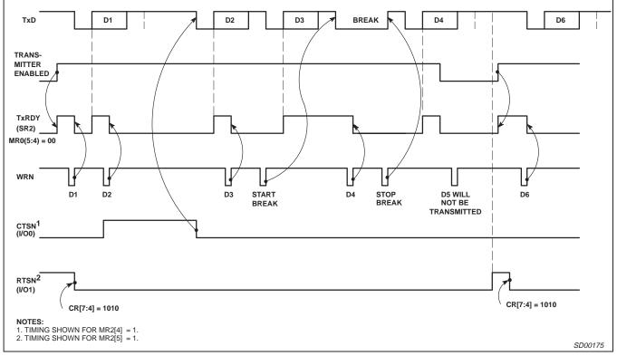
Figure 16. Transmitter Data Timing
