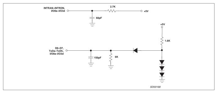
Figure 9. AC Test Conditions on Outputs
