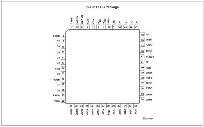
Figure 1. Pin configuration
