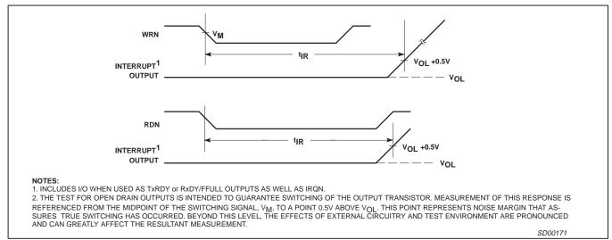
Figure 12. Interrupt Timing
