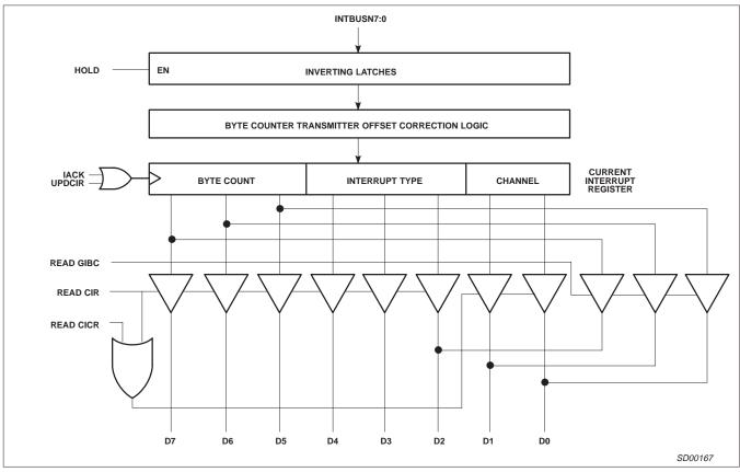
Figure 8. Current Interrupt Register Logic
