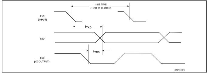
Figure 14. Transmit Clock Timing
