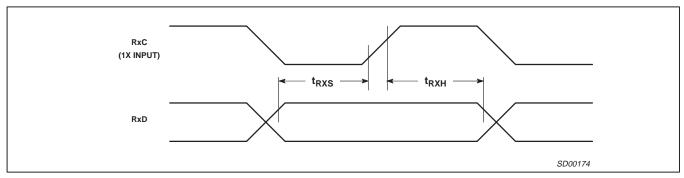
Figure 15. Receive Clock Timing
