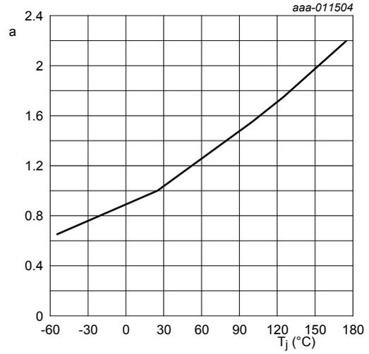
$$a = \frac{R_{DS(on)}}{R_{DS(on)}(25^\circ C)}$$
