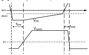
Figure 2: Turn-On and Turn-Off delay
