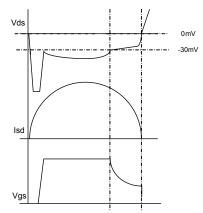
Figure 3: Synchronous Rectification Operation at Heavy Load
