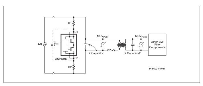
Figure 3. Placement Options of MOV and  $C_{EXT}$
