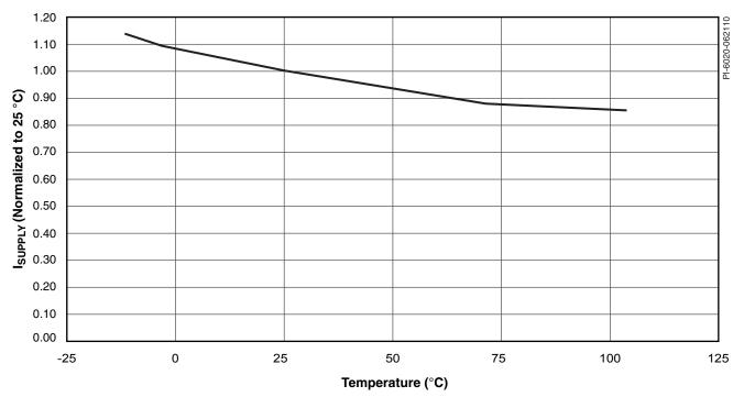
$\textit{Figure 5.} \quad \textit{I}_{\textit{SUPPLY}} \textit{vs. Temperature.}$
