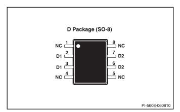
Figure 2. Pin Configuration.
