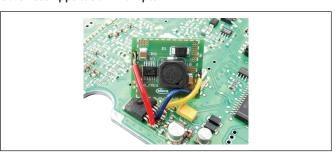
The buck-core is available as stand-alone 3-wire PCB. It can be easily applied in any application as replacement. Core characterization report and layout data (gerber-file) are available.
