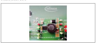
The buck-core is designed with the aim to be reproduced in customer applications (see dashed area in the right picture).
