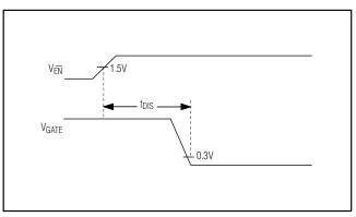
Figure 4. Disable Timing Diagram
