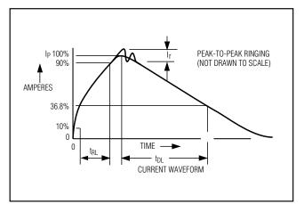
Figure 9. Human Body Model Current Waveform
