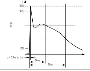
Figure 11. IEC 61000-4-2 ESD Generator Current
