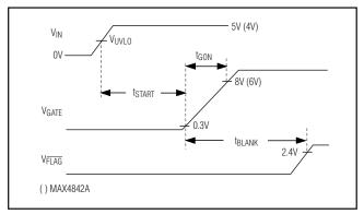
Figure 1. Startup Timing Diagram
