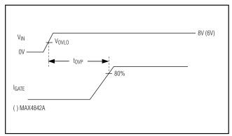
Figure 3. Power-Up Overvoltage Timing Diagram
