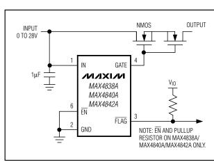
Figure 7. Back-to-Back External MOSFET Configuration
