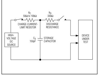
Figure 10. IEC 61000-4-2 ESD Test Model
