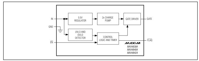
Figure 5. Functional Diagram
