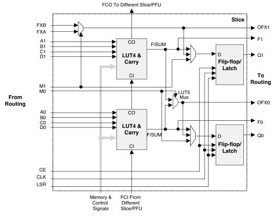
For Slices 0 and 1, memory control signals are generated from Slice 2 as follows:
