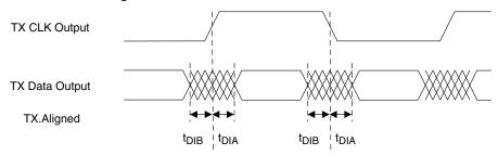
Figure 3-8. Transmitter TX.CLK.Centered and MEM DDR Output Waveforms
