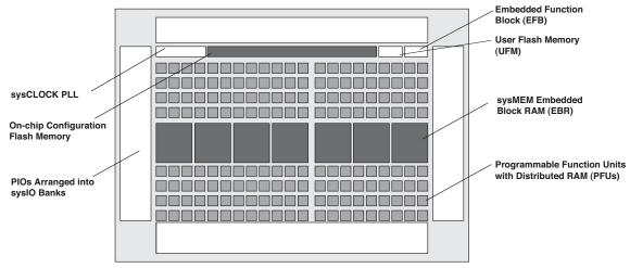
Note: MachXO2-256, and MachXO2-640/U are similar to MachXO2-1200. MachXO2-256 has a lower LUT count and no PLL or EBR blocks. MachXO2-640 has no PLL, a lower LUT count and two EBR blocks. MachXO2-640U has a lower LUT count, one PLL and seven EBR blocks.
