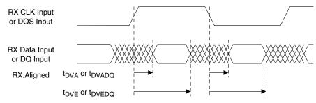
Figure 3-6. Receiver RX.CLK.Centered Waveforms
