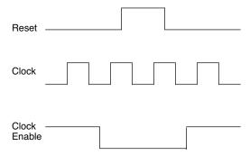
If all clock enables remain enabled, the EBR asynchronous reset or GSR may only be applied and released after the EBR read and write clock inputs are in a steady state condition for a minimum of 1/f<sub>MAX</sub> (EBR clock). The reset release must adhere to the EBR synchronous reset setup time before the next active read or write clock edge.
