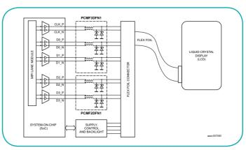
Using PCMFDFN1 in a MIPI DSI display interface
