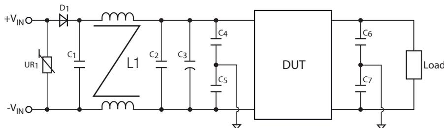
It is recommended to add UR1, D1 and C1 in railway application. C1, L1, C2 and C3 can be modified for required EMI standards. To meet EN61000-4-2, module case should be earth grounded. We offer independent case pin option on request, the location is upon pin 1.
