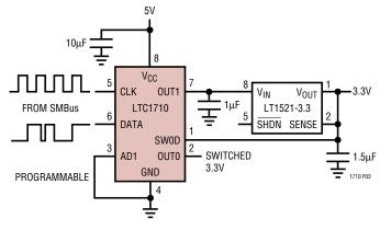
Figure 3. Low Dropout Regulator Switching a 3.3V/300mA Supply
