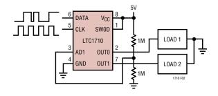
Figure 2. The LTC1710 Programmed with Address 1011001
