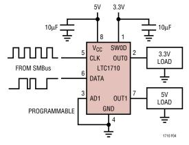
Figure 4. The LTC1710 Switching Two Different Voltage Loads
