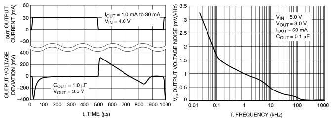
Figure 11. Load Transient Response
