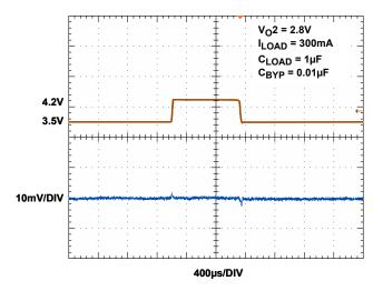
FIGURE 14. LINE TRANSIENT RESPONSE, 2.8V OUTPUT
