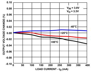
FIGURE 2. OUTPUT VOLTAGE CHANGE vs LOAD CURRENT
