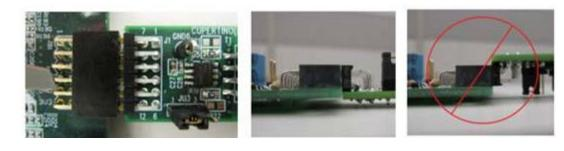
Figure 2. Pmod™ Connector Alignment
