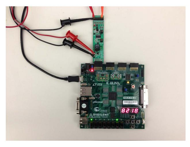
Figure 1. Corona Board Connected to Nexys 3 Development Kit
