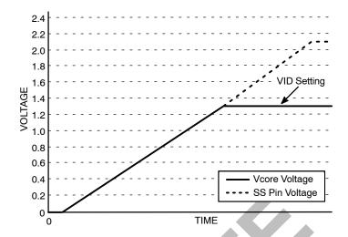
Figure 9. Typical VR10 Soft-Start Sequence to Vcore = 1.3 V
