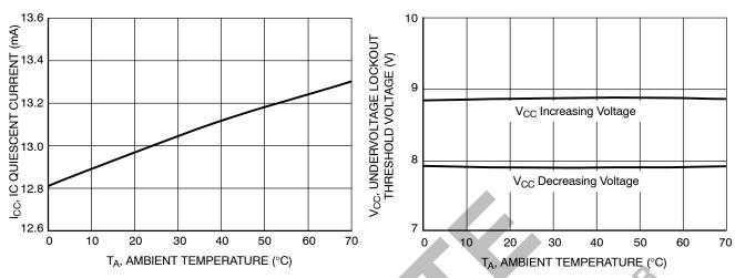
Figure 6. IC Quiescent Current vs. Ambient **Temperature**
