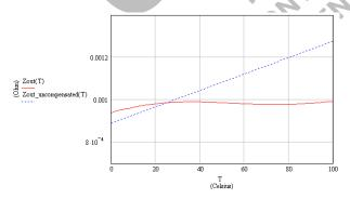
Figure 22. Uncompensated and Compensated Output Impedance vs. Temperature
