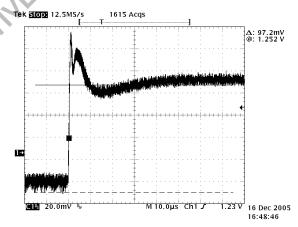
Figure 12. Typical Load Release Event
