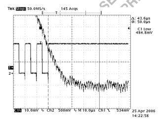
Figure 15. Dynamic VID Settling Time Falling
