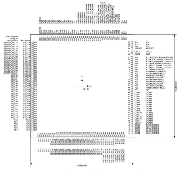
Figure 1.3.2.1 S1C17W34/W35/W36 Pad Configuration Diagram (Chip)
