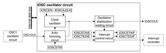
Figure 2.3.3.1 IOSC Oscillator Circuit Configuration
