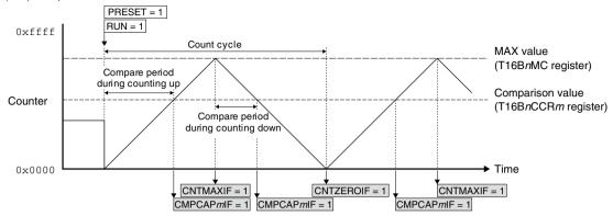
(Note that the T16BnINTF.CMPCAPmIF/CNTMAXIF/CNTZEROIF bit clearing operations via software are omitted from the figure.) Figure 15.4.3.1 Operation Examples in Comparator Mode
