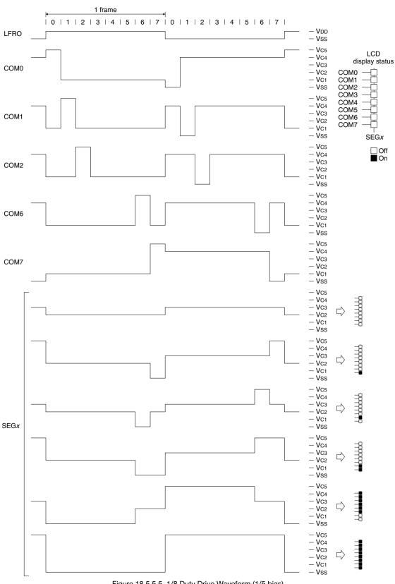
Figure 18.5.5.5 1/8 Duty Drive Waveform (1/5 bias)
