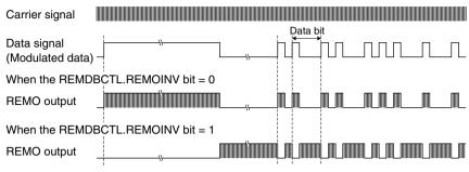
Figure 17.4.3.1 REMO Output Waveform Example
