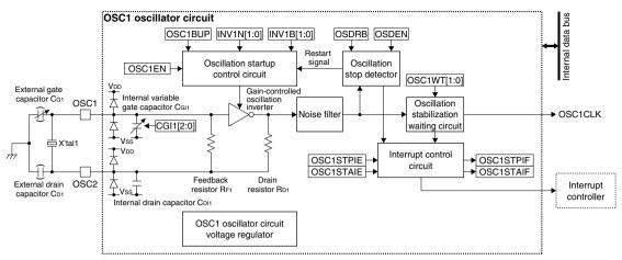
Figure 2.3.3.2 OSC1 Oscillator Circuit Configuration
