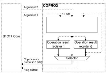
Figure 22.6.1 Data Path in Operation Result Read Mode
