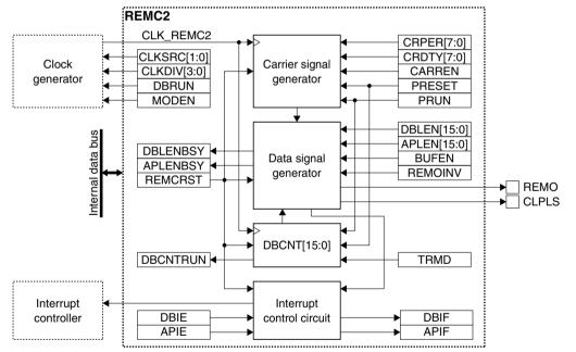
Figure 17.1.1 REMC2 Configuration
