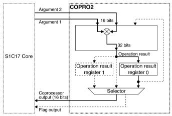
Figure 22.3.1 Data Path in Multiplication Mode
