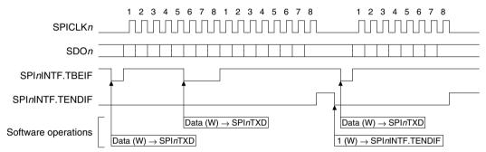
Figure 13.5.2.1 Example of Data Sending Operations in Master Mode (SPInMOD.CHLN[3:0] bits = 0x7)
