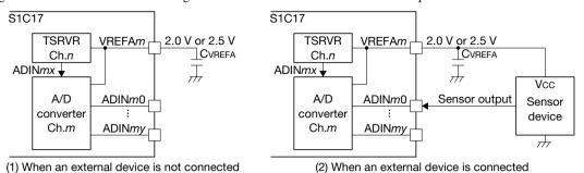
Figure 21.2.2.1 Connections between TSRVR and External Components
