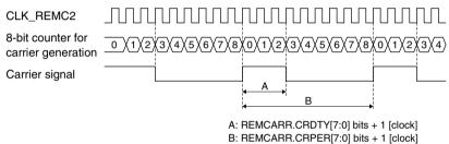
Figure 17.4.3.2 Example of Carrier Signal Generated
