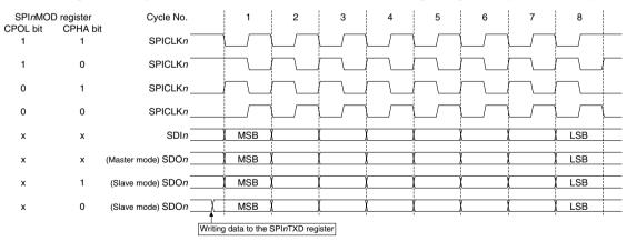
Figure 13.3.3.1 SPI Clock Phase and Polarity (SPInMOD.LSBFST bit = 0, SPInMOD.CHLN[3:0] bits = 0x7)
