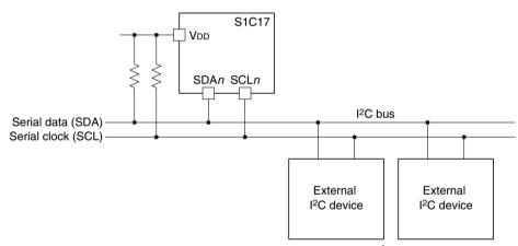
Figure 14.2.2.1 Connections between I2C and External I2C Devices
