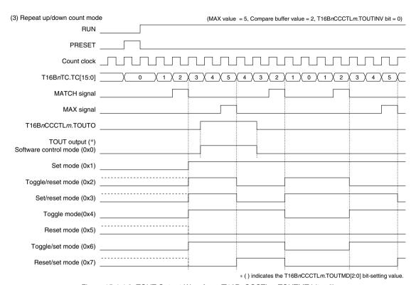
Figure 15.4.4.2 TOUT Output Waveform (T16BnCCCTLm.TOUTMT bit = 0)
