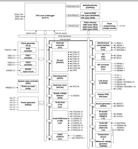
Figure 1.2.1 S1C17W34/W35/W36 Block Diagram
