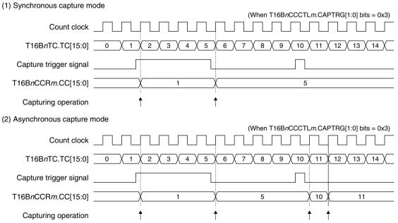
Figure 15.4.3.4 Synchronous Capture Mode/Asynchronous Capture Mode
