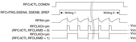
Figure 19.4.5.1 CR Oscillation Clock (RFCLK) Waveform
