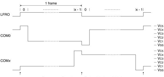
Figure 18.7.1 Frame Interrupt Timings (1/x duty, 1/5 bias)
