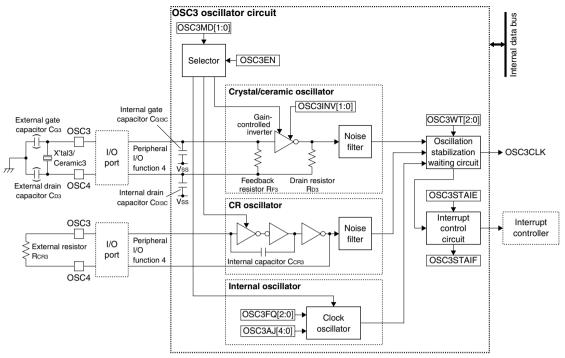
Figure 2.3.3.3 OSC3 Oscillator Circuit Configuration
