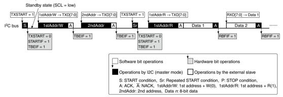
Figure 14.4.4.2 Example of Data Transfer Starting Operations in 10-bit Address Mode (Master Mode)
