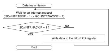
Figure 14.4.5.2 Slave Mode Data Transmission Flowchart
