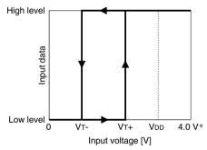
(\* For over voltage tolerant fail-safe type port)
