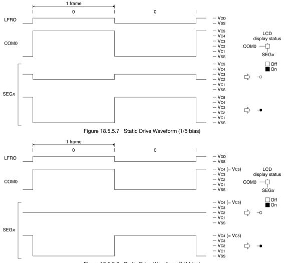
Figure 18.5.5.8 Static Drive Waveform (1/4 bias)
