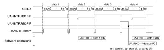
Figure 12.5.3.1 Example of Data Receiving Operations
