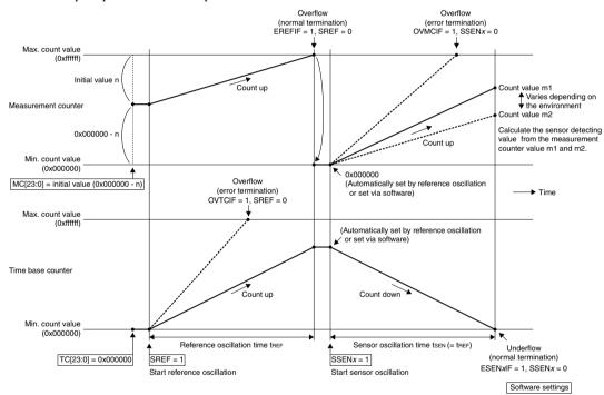
Figure 19.4.4.1 Counter Operations During Reference/Sensor Oscillation
