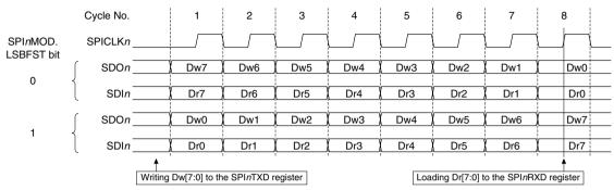
Figure 13.4.1 Data Format Selection Using the SPInMOD.LSBFST Bit (SPInMOD.CHLN[3:0] bits = 0x7, SPInMOD.CPOL bit = 0, SPInMOD.CPHA bit = 0)
