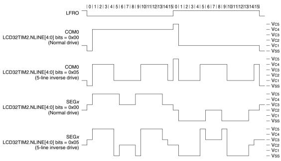
Figure 18.5.7.1 1/16 Duty (1/5 bias) Normal Drive Waveform and 5-line Inverse Drive Waveform
