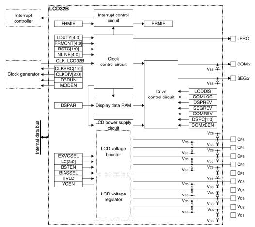
Figure 18.1.1 LCD32B Configuration
