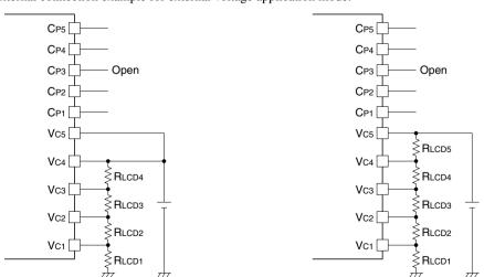
When 1/4 bias is selected (LCD8PWR.BIASSEL bit = 1) When 1/5 bias is selected (LCD8PWR.BIASSEL bit = 0) Figure 18.4.2.1 External Connection Example for External Voltage Application Mode (Resistor Divider)
