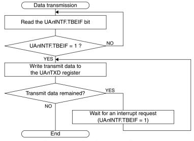
Figure 12.5.2.2 Data Transmission Flowchart
