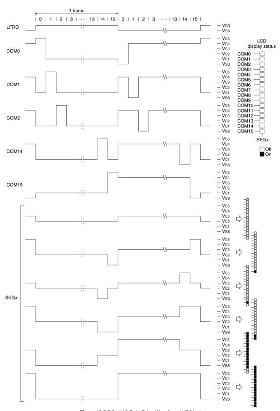
Figure 18.5.5.3 1/16 Duty Drive Waveform (1/5 bias)
