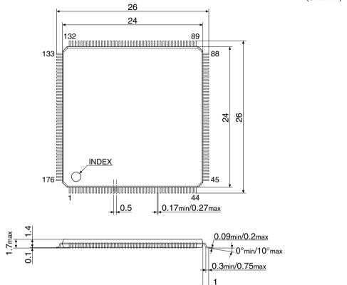
Figure 25.1 QFP21-176pin Package Dimensions
