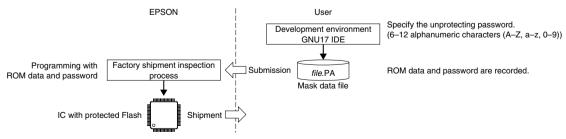
Figure 3.3.5.1 Shipment of IC with ROM Data Programmed and Flash Security Function Setting Flow
