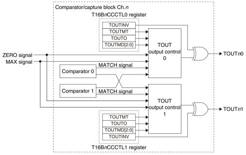
Figure 15.4.4.1 TOUT Output Circuits (Circuits 0 and 1)
