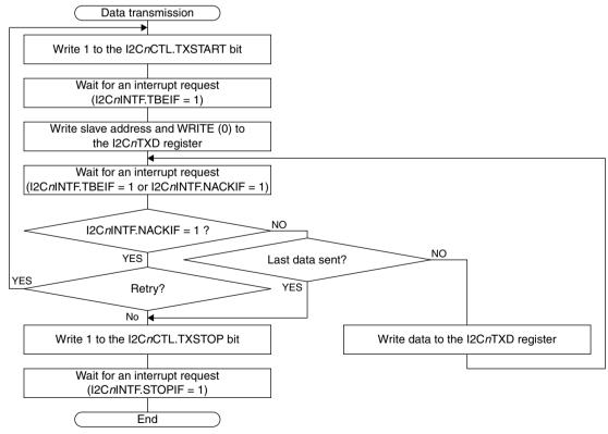
Figure 14.4.2.2 Master Mode Data Transmission Flowchart
