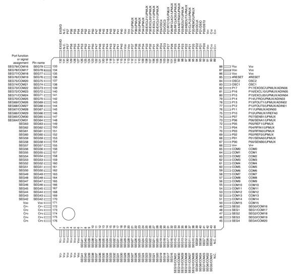
Figure 1.3.1.1 S1C17W34/W35/W36 Pin Configuration Diagram (QFP21-176pin)
