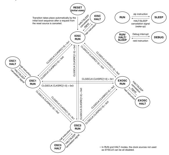
Figure 2.4.2.1 Operating Mode-to-Mode State Transition Diagram
