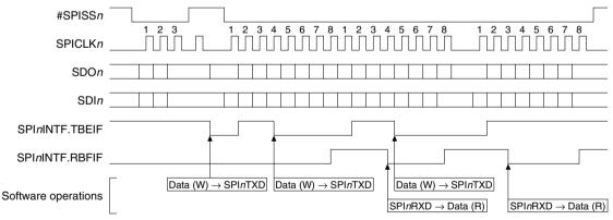
Figure 13.5.5.1 Example of Data Transfer Operations in Slave Mode (SPInMOD.CHLN[3:0] bits = 0x7)
