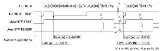
Figure 12.5.2.1 Example of Data Sending Operations
