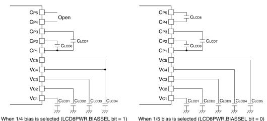
Figure 18.4.1.1 External Connection Example for Internal Generation Mode
