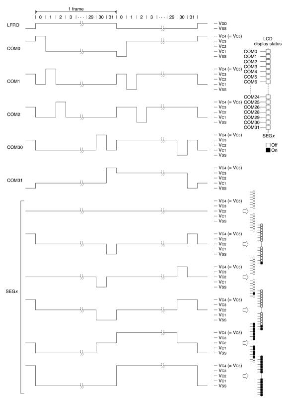
Figure 18.5.5.2 1/32 Duty Drive Waveform (1/4 bias)
