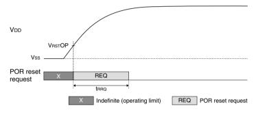
**Note**: When performing a power-on-reset again after the power is turned off, decrease the V<sub>DD</sub> voltage to V<sub>RST</sub>OP or less.
