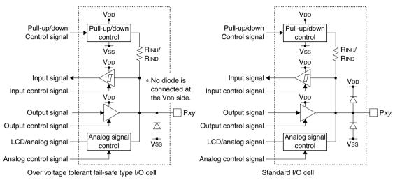
Figure 6.2.1 I/O Cell Configuration
