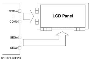
Figure 18.2.2.1 Connections between LCD32B and an LCD Panel
