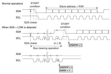
Figure 14.4.8.1 Automatic Bus Clearing Operation
