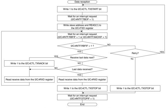
Figure 14.4.3.2 Master Mode Data Reception Flowchart
