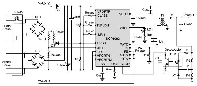
Figure 2. Isolated Fly-back Converter with Rear Auxiliary Support
