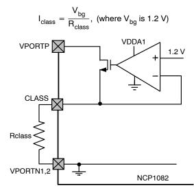
Figure 8. Classification Block Diagram
