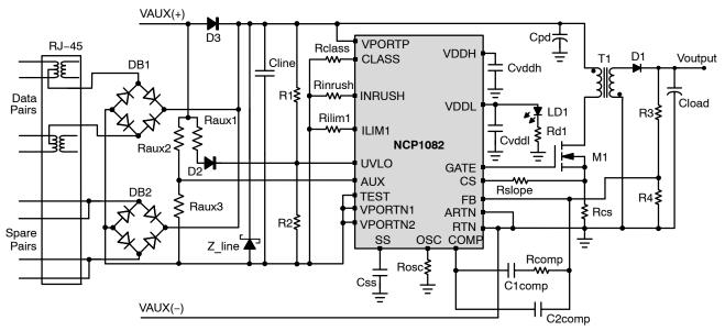
Figure 3. Non-Isolated Fly-back Converter with Rear Auxiliary Support
