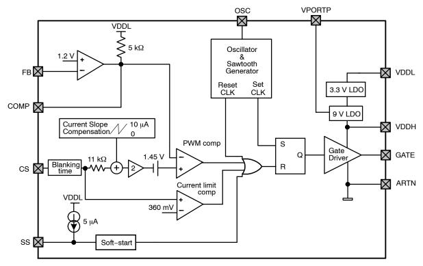
Figure 14. DC–DC Controller Block Diagram
