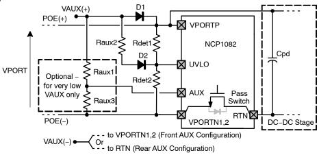
Figure 11. Front and Rear Auxiliary Supply Input with Support for Very Low Input Voltages
