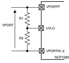
Figure 10. External UVLO Configuration
