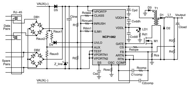
Figure 5. Non–Isolated Forward Converter with Rear Auxiliary Support
