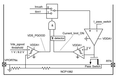
Figure 13. Inrush and Ilim1 Selection Mechanism
