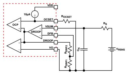
FIGURE 9. EQUIVALENT MODEL FOR DROOP CIRCUIT USING DISCRETE RESISTOR CURRENT SENSING
