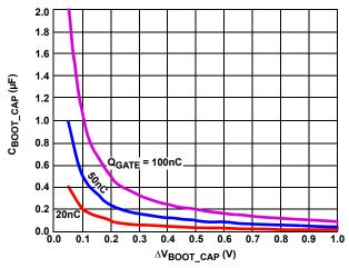
FIGURE 7. BOOTSTRAP CAPACITANCE vs BOOT RIPPLE VOLTAGE
