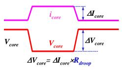
FIGURE 10. DESIRED LOAD TRANSIENT RESPONSE WAVEFORMS
