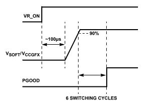
FIGURE 4. ISL6263 START-UP TIMING
