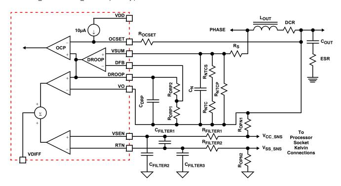
FIGURE 5. SIMPLIFIED VOLTAGE DROOP CIRCUIT WITH GPU SOCKET KELVIN SENSING AND INDUCTOR DCR CURRENT SENSING
