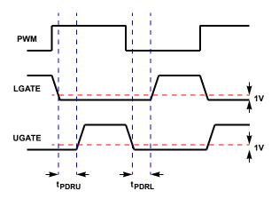
FIGURE 6. GATE DRIVER TIMING DIAGRAM
