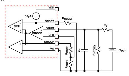
FIGURE 8. EQUIVALENT MODEL FOR DROOP CIRCUIT USING INDUCTOR DCR CURRENT SENSING
