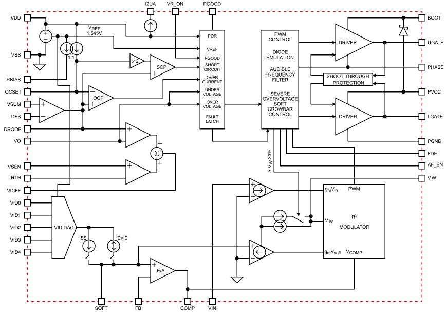
FIGURE 1. SIMPLIFIED FUNCTIONAL BLOCK DIAGRAM OF THE ISL6263
