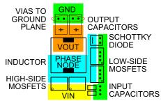
FIGURE 13. TYPICAL POWER COMPONENT PLACEMENT
