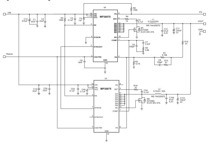
Figure 7—Two Phase Operation
