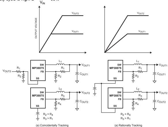
Figure 6—Output Voltage Tracking
