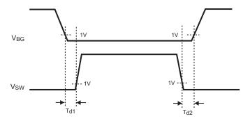
Figure 1—Gate Drive Non-Overlap Time Diagram
