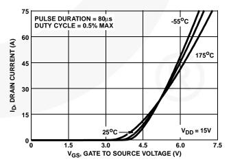
FIGURE 8. TRANSFER CHARACTERISTICS
