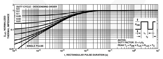
FIGURE 3. NORMALIZED MAXIMUM TRANSIENT THERMAL IMPEDANCE
