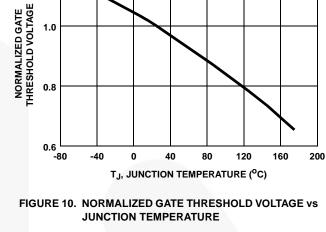
$V_{GS} = V_{DS}, I_D = 250 \mu A$
