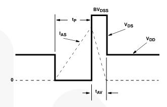
FIGURE 15. UNCLAMPED ENERGY WAVEFORMS
