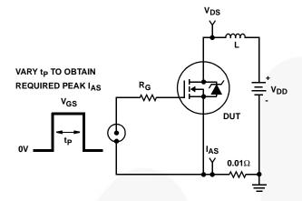
FIGURE 14. UNCLAMPED ENERGY TEST CIRCUIT
