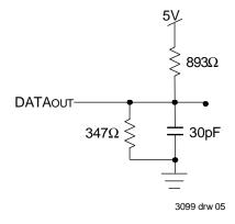
Figure 1. AC Output Test Load
