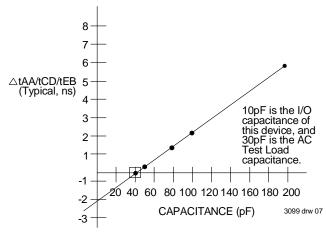
Figure 3. Lumped Capacitance Load Typical Derating Curve
